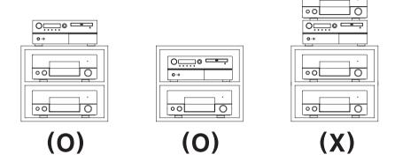
Placement of this system on a well-ventilated area (good intake of cold air and release of hot air) allows efficient cooling of computer components even in low RPM mode, for ultra quiet operation. The noise level of the power supply (main factor of noise emission) will also significantly decrease due to better cooling efficiency.
