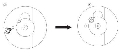
Unscrew the HDD Lock Bar's Fixing Screw from the HDD Chassis with a Phillips screwdriver.
