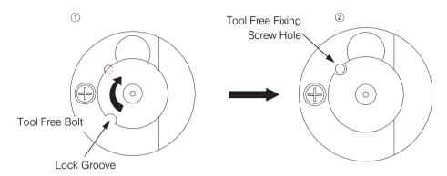
Align the Lock Groove of the HDD Lock Bar with the Fixing Screw Hole.
