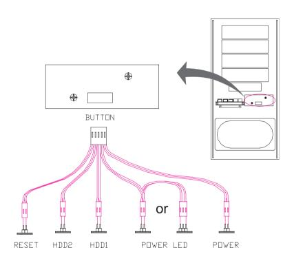
\* Improper connection of the Power LED and HDD LED can lead to LED malfunction.
