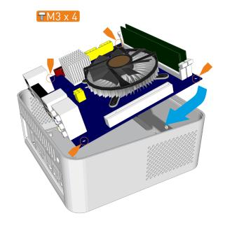
Carefully lower the motherboard into the chassis, with the I/O port side leading so that the ports can fit into the I/O shield.
