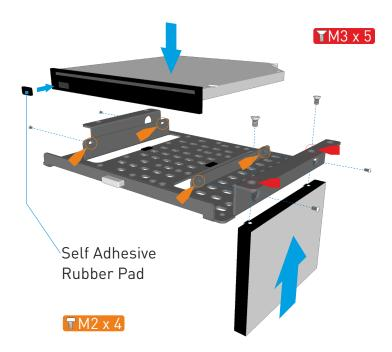
Before fitting the slot loading drive, affix a self adhesive rubber pad to the drives eject button (included in the accessory bag). Mount the slot loading drive using 4 screws, 2 either side, and adjust is position to ensure correct operation of the eject button. With left side eject buttons, 2 pads may be required.
