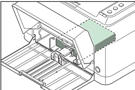
When using A6 paper, load the paper as shown in the illustration.
