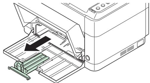
When using A6 paper, attach the stopper.
