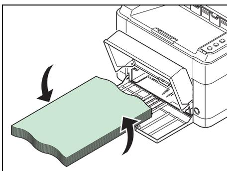
When the paper feed fails because the edge of the paper is wavy, turn it upside down and load it again.
