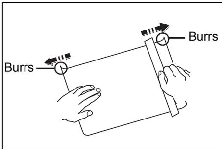
Fan the stack of paper and align the edges before loading them in the paper source. Some types of paper have rough edges on the back (those are created when the paper is cut). In this case, put the paper on a flat place and rub the edges once or twice with, for example, a ruler to smooth them. Feeding rough edged paper may cause paper jams.
