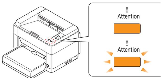
**Note** If the indicators light or flash repeatedly in manners not described above, a service error has probably occurred. Switch off the printer power switch, unplug the power cord, and then plug the power cord back in and switch on the power switch. This may clear the error. If the error is not cleared, contact your service technician.
