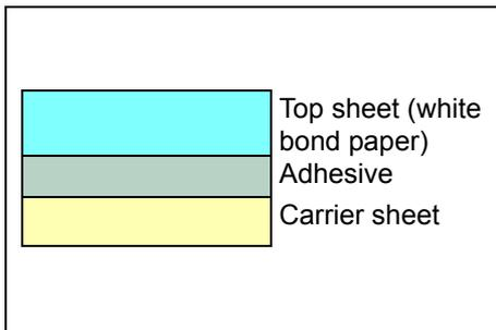
Label paper has a structure comprising of three layers, as shown in the diagram. The top sheet is printed on. The adhesive layer consists of pressure-sensitive adhesives. The carrier sheet (also called the linear or backing sheet) holds the labels until used. Due to the complexity of its composition, adhesive-backed label paper is particularly likely to give printing problems.
