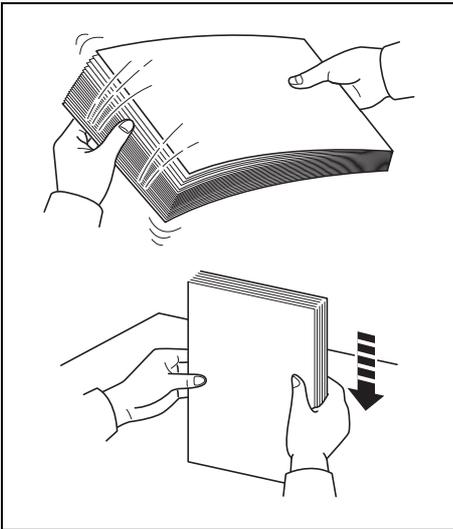
After removing paper from the packaging, fan through the sheets to separate them prior to loading.
