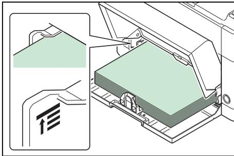
If an excessive amount of thick paper is loaded in the cassette, it may not be fed. In that case, reduce the number of sheets to be loaded.
