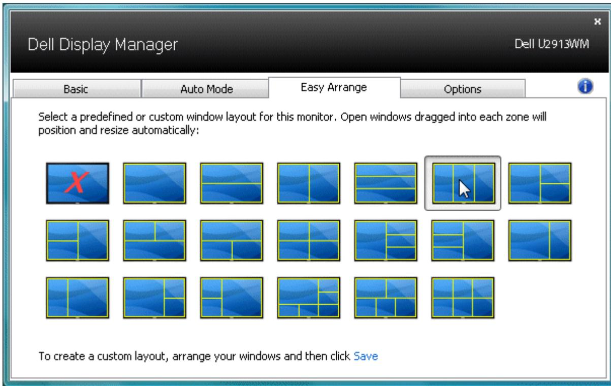
To create a custom window layout, first size and position up to 10 windows on the desktop and then click the **Save** link in **Easy Arrange**. The size and position of the windows is saved as a custom layout and the custom layout icon is created.
