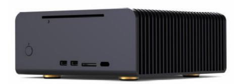
The FC8 has three single USB headers that need connecting to your motherboard, two for the dual USB slots and one for the card reader.
