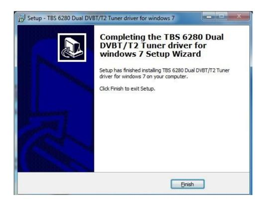
To verify if driver was correctly installed, you could check computer device manager. You will see "TBS 6280 DVB-T2/T BDA Tuners" under the "Sound, video and game controllers" bar of "Device Manager" if the driver is correctly installed.
