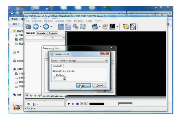
After you have completed the settings, you could click "Scan" or "Manual Scan" under "Channels" menu to search for channels. If you don't know the exact frequency, Auto Scan is recommended.
