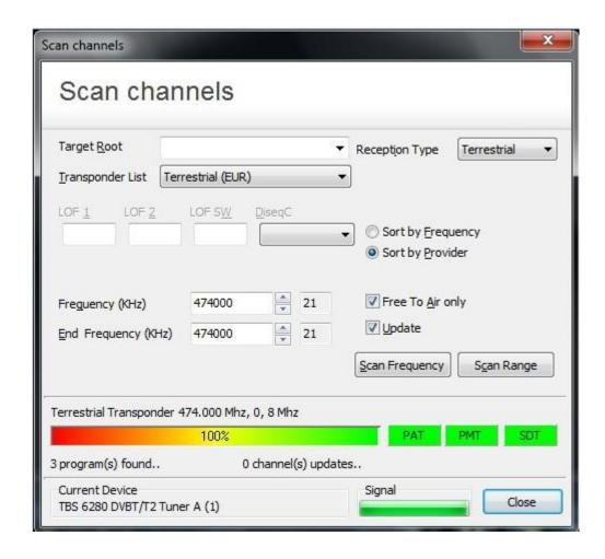
After scan is completed, the found program numbers will be shown and the program list will be automatically saved. You can close the "Scan channels" window.
