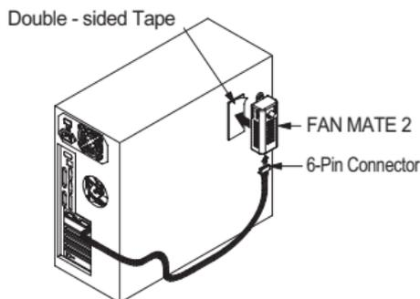
Pull the 6-pin connector out of the system through the back and connect it to FAN MATE 2, which should be installed on the case using the included double-sided tape (①).
