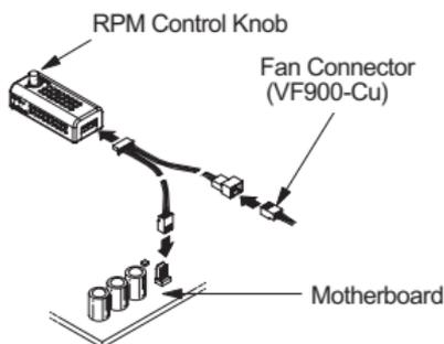
Connect the appropriate 3-pin connector on the cable to the motherboard fan header and the VF900-Cu fan connector.
