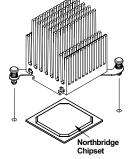
4. Clean the surface of the Northbridge 5. Insert the push pins into the mounting holes on the motherboard and ensure they remain firmly in place.
